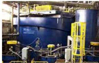
Our flotation tanks universal design, can accommodate self-aspirated WEMCO® mechanisms, or forced-air DORR-OLIVER® mechanisms. Thus allowing our clients to achieve greater flexibility and more control over processing of coarse and fine particles for maximum recovery.
