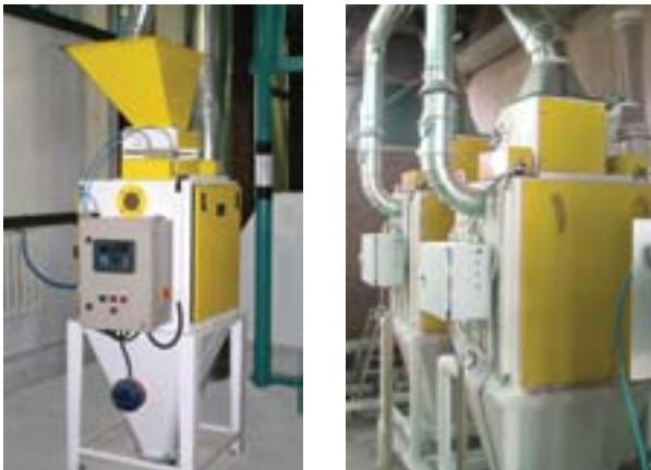
Automatic weighers are used to weigh granule and powdered materials during the continuous flows at flour mills, cereal processing and storage plants, cereal cleaning systems, cereal storage silos and in port cereal storage facilities.
