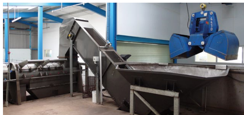
TS3096 Turbo Separator system with caterpillar in-feed conveyor capable of separating up to 10 tonnes per hour of mixed packaged food waste
