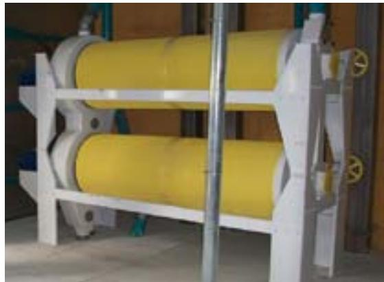
Trieurs are used to separate the round particles smaller than wheat kernels, broken wheat kernels and longer particles bigger than wheat kernels.
