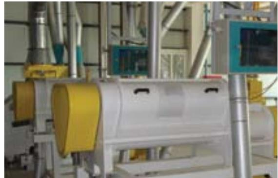
Intensive dampeners are used to moisturize the grains to a sufficient moisture content in the mill plants to ease the processing performances with economic usage of energy, increasing usage life of the equipments.
