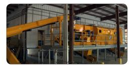
The CBI AirMax material separator component is versatile for C&D recycling, glass recycling, mulch cleanup, compost cleanup and automotive fluff recycling. The AirMax requires minimal power from four motors totaling 32 HP.
