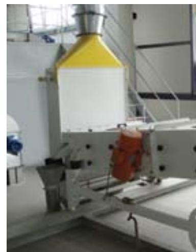
Aspiration channels are used to remove and clean light impurities and foreign materials from cereals by means of air. They can be used by the combination of either scourers (with vibro-motor) or separators (without vibro-motor).
