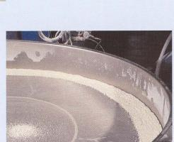
MINIMUM SCREEN BLINDING for all separation processes is achieved through the use of and the combination of several techniques. The vibration of the Separator, the use of sliders, the use of bouncing balls, the use of ultra-sonics, the use of water sprays, the use of wipers, and last but not least, the use of good well tensioned screens.
