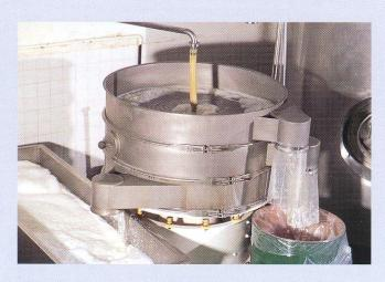
**NO TRANSMITTED VIBRATION** was a need for a dairy and juice producer. The AMKCO is mounted on a portable stand, easily moveable to different locations for different products. The various locations have floors that are not always level. Quick and easy shims under the legs keep the screen level for good separation.
