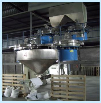
From a Milling flour factory. They choose MCL-500 with 24# (mesh size). The reference capacity is 300 KG/h (each one). Their target is to remove impurity of flour. The contact part is stainless steel 304(GMP standard). The mesh material is Stainless steel 304.
