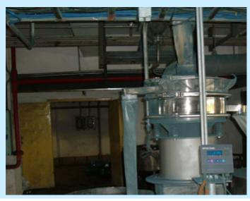
From a chemical factory. Their target is to dewater from the granules. They choose MCL-800-1 with 100 mesh sieve. The reference capacity is 300 kg/h. The contact part is stainless steel 304(GMP standard). The mesh material is Stainless steel 304.
