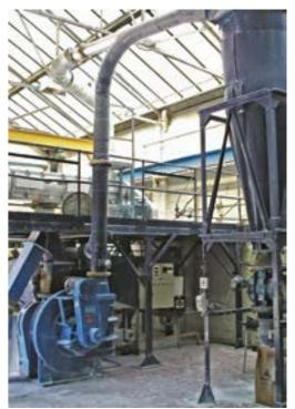
The 8A Dryer-Pulveriser in Atritor's test facility
