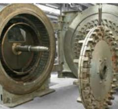
Fitting the rotor in a 20A Dryer-Pulveriser
