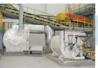
An 18A Dryer-Pulveriser and gas-fired air heater for processing precipitated calcium carbonate (PCC)
