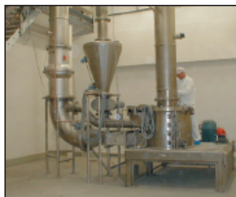
DCM 800 classifier mill is one of a pair processing food ingredients
