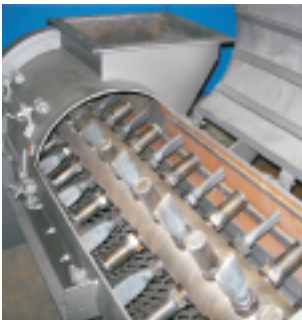
Atritor-Scott Turbo Separator, Separates Product from Packaging for Recycling or Disposal.
