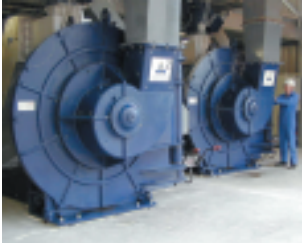
"A" & "B" Series Atritor Dryer-Pulverisers for Chemicals & Minerals.
