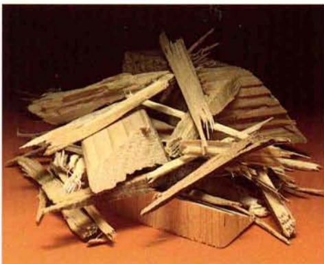
Pallet chippers and ordinary hogs leave large splinters and coarse chunks - not suitable for resale.
